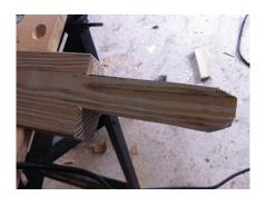
(either end of the bit of wood you want to remove), then use a jigsaw and/or chisel to remove the extra wood and smooth it down.
