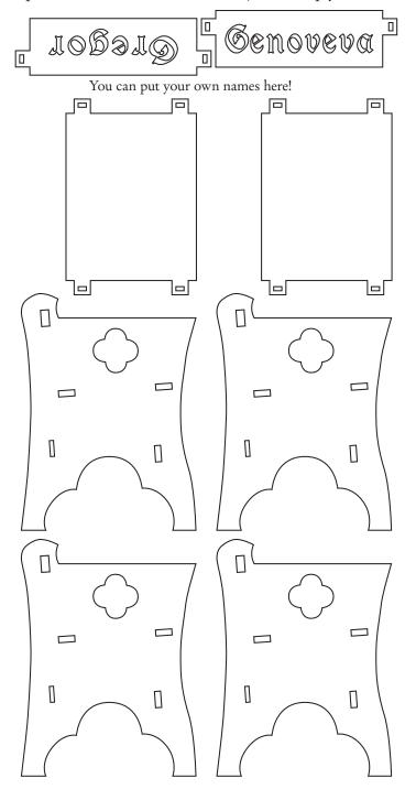
Cut these pieces from one 4'x8' sheet of 1/2" thick plywood then glue together (align tops).
