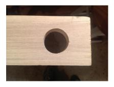
4. Now assemble your rack by placing cris-crossing the tops of two boards and putting the larger dowel through both holes, then repeat with the other two boards on the other end of the dowel. Now slide the smaller dowels into the holes at the bottom of the legs. (You may need to tap the dowels and/ or boards to get them all to slide through the holes — you want it to be pretty snug for stability.)
