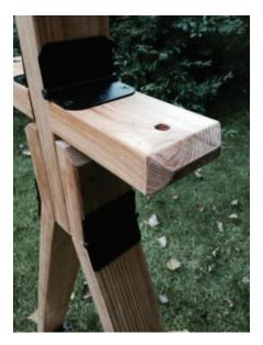
Step 3. Take board A, find the exact center of the board lengthwise, and drill a hole all the way through the board using the 1/2" bit. On one side of this board, use the 11/2" spade bit to create a recess about 3/4" deep around the hole you just drilled. (This will accommodate your washer and wing nut.)
